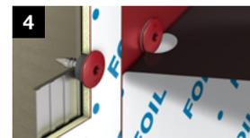
**Installation of the XT system:** 1. Insert XT centring grommet into pre-punched facade panel; 2. Rotate XT centring grommet with LT-XT-Tool in order to cut the protective film; 3. Fasten LT-XT screw with LT-XT-Tool in support profile; 4. Remove protective film gently over the fixing point
